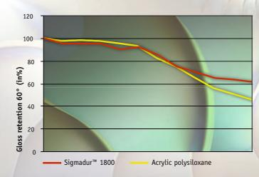
As can be seen from the WOM exposure SigmaDur™ 1800 outperforms Generally acrylic polysiloxane technology has not proved to provide a risk free technology for 15-20 years service. When the build up of internal stress (ASTM D6991-05) of SigmaDur™ 1800 has been determined and compared with acrylic polysiloxane available in the market the following has been observed.
