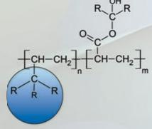
The binder is styrene free, which will result in a longer durability when exposed to UV:
