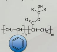
Unfortunately the styrene in this building block is the part where we can find the weakness when it is exposed to ultraviolet (UV), which is part of daylight. Styrene is a weakness when binder is exposed to UV because of the following reasons:
