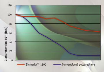
Because SigmaDur™ 1800 is a durable finish that is designed for a durability up to 20 years it is in the arena with acrylic polysiloxane. The comparison in accelerated tests (WOM, ISO 4892-2) with conventional polysiloxane is as following.
