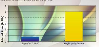
SigmaDur™ 1800 builds up 6 times less internal stress than an acrylic polysiloxane that is available in the market and hence is less sensitive for over application and thus cracking. This can clearly be observed from mandrel testing (ISO 1519).
